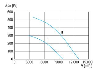
I Characteristic curve for speed I II Characteristic curve for speed II
