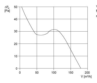
V = 230 or 24 Vf = 50 Hz n = 2600 min<sup>-1</sup>
