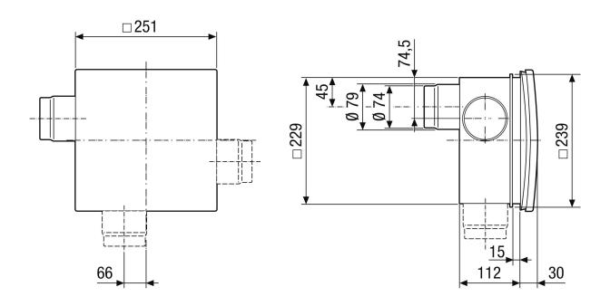
Fan insert ER ... E with ER-UP/GH recess-mounted housing and second room connection
