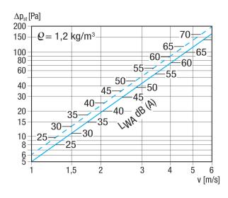
Dashed line: Pressure loss, drawing in Solid line: Pressure loss, pushing
