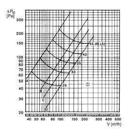
① 20 revolutions, 1 mm stroke height per revolution A: 1/4 open, B: 1/2 open, C: 3/4 open, D: open all the way
