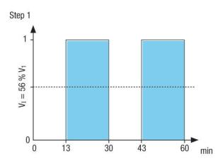
Interval switch for step 1 17 min to switch on 13 min to switch off
