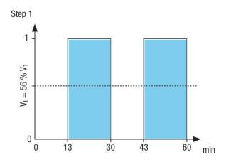
Interval switch for step 1 17 min to switch on 13 min to switch off
