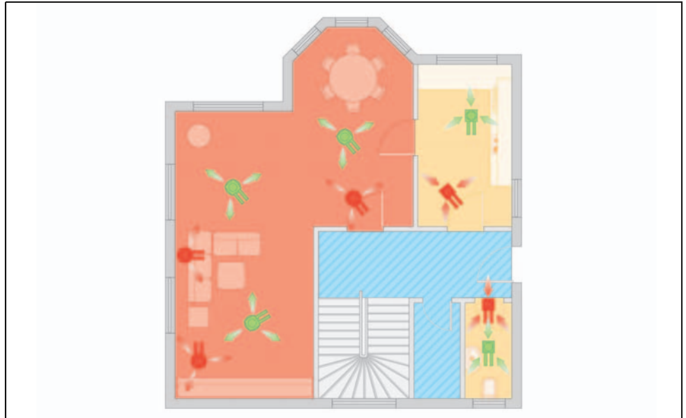
Green: Correct positioning of the supply / exhaust air openings / Red: Incorrect positioning of the supply / exhaust air openings
