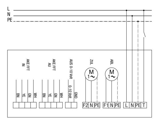
EA – Exhaust air SA – Supply air OUT – Output OSA – Outer
