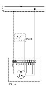
DS 3N - 3-step switch Terminals 1-4 are the motor's windings. Assignment of terminals by way of example: Minimum speed (terminal 1) is not used here.
