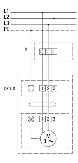
For right-hand operation, swap 2 phases on fan connection b on site
