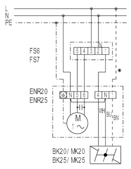
FS 6 - Step switch for (2-speed, air extraction or ventilation)
