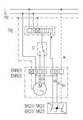
TRE - 5-step transformer (on/off, 5-speed)
