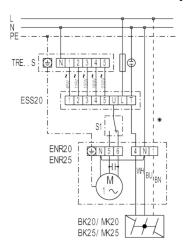
TRE - 5-step transformer, control cabinet installation
