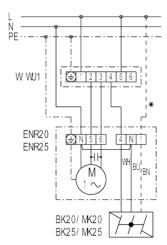
W 1 - Reversing switch (air extraction or ventilation), surface mounted WU 1 - Reversing switch (air extraction or ventilation), recessed mounted \* - duct only for MK... shutter
