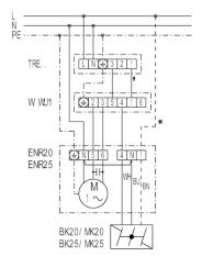
TRE - 5-step transformer (on/off, 5-speed)
