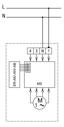
MS - motor control Connection is made in the housing
