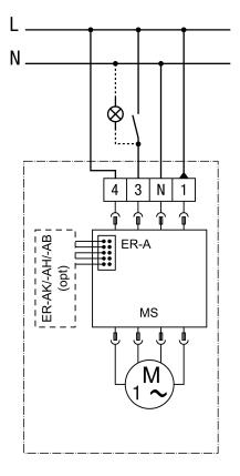
opt - optional MS - motor control Full load can be switched with permanent base load Connection is made in the housing
