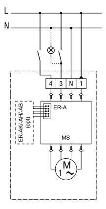
opt - optional MS - motor control Base and full load can be switched Connection is made in the housing
