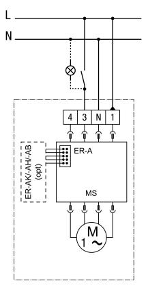
opt - optional MS - motor control Full load can be switched, no base load operation Connection is made in the housing
