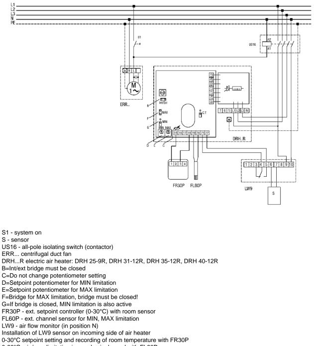
0-60°C min/max limitation in supply air channel with FL60P
