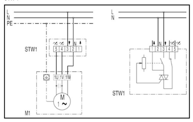
STW speed controller Terminal 1 additional connection (without control) M1 fan (right-hand/left-hand operation)
