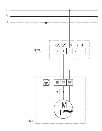
STW 1 - Speed controller Terminal 1 - Additional connection (without control) M1 - Fan (right-hand / left-hand operation)
