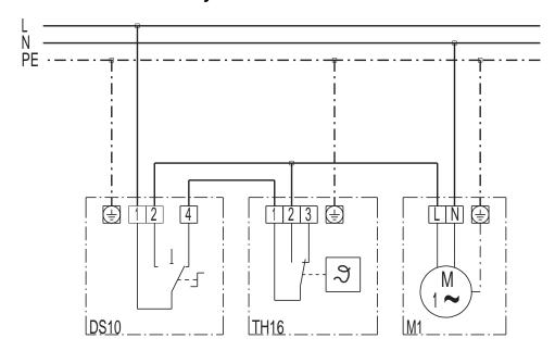
DS 10 - rotary switch 2 - continuous operation 4 - normal operation TH 16 - thermostat
