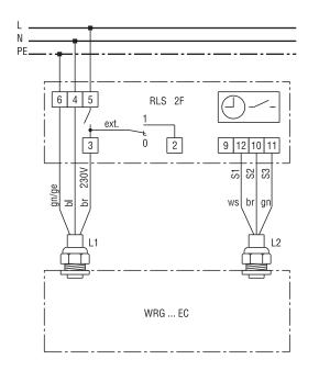
WRG 180 EC ventilation unit with ERH electrical air heater
