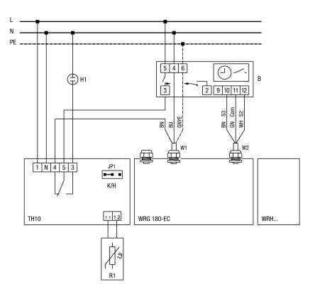
TH 10 - thermostat with R1 temp.sensor R1 - temperature sensor / installation in the supply air channel ahead of the WRH JP1 - plug jumper JP1 on operating mode "K". Relay switches WR 180 EC off as the temperature drops. WRG 180 EC - ventilation unit B - room air control RLS 2 F (operator unit with timer) W1 - 230 V AC connecting cable W2 - control cable for room air control WRH... - water air heater
