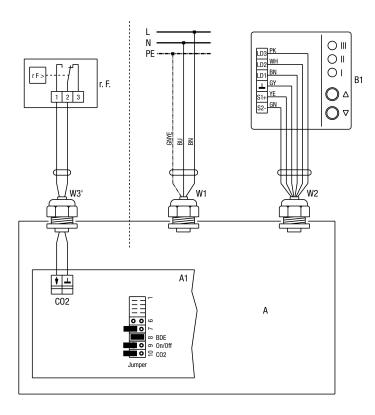
Connection of hygrostat with potential-free contact. If the potential-free contact in the hygrostat closes due to room dampness, the ventilation unit is set to LS3 regardless of the ventilation level set. Once the dampness has been removed from the room (contact in hygrostat opens), the ventilation unit switches back to the ventilation level previously set.
