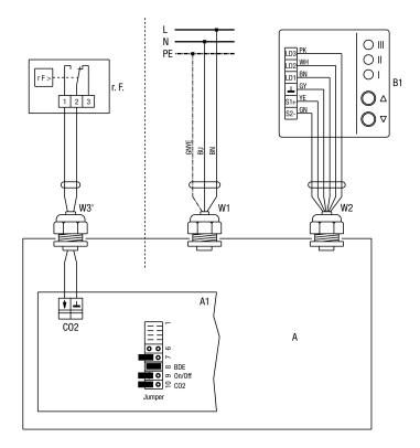
Connection of hygrostat with potential-free contact. If the potential-free contact in the hygrostat closes due to room dampness, the ventilation unit is set to LS3 regardless of the ventilation level set. Once the dampness has been removed from the room (contact in hygrostat opens), the ventilation unit switches back to the ventilation level previously set.
