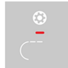
Fig. 1: Example of an operating unit fault with 3 illuminated elements → Fault/failure CO2 combi sensor.
