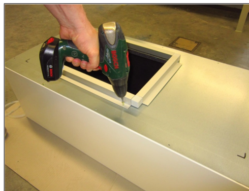
10. Use the four M8 x 25 mm screws supplied to permanently screw down the terminal box to the unit.
