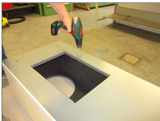
9. Screw the two connection frames to the terminal box (16 x drilling screws 3.5 x 13 mm).
