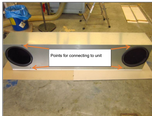
10. Use the four M8 x 25 mm screws supplied to permanently screw down the terminal box to the unit.
